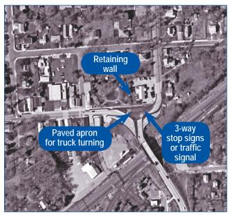
Depiction of a possible reconfiguration of the MD 564 bridge to create a safer T-intersection.
